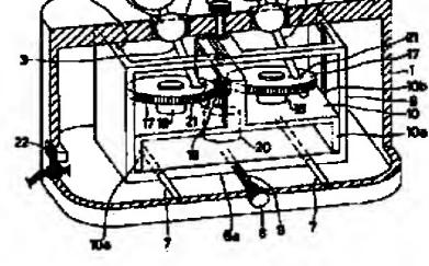
disks rotated horizontally. Both disks are provided on an elevating support plate, and the support plate is installed in a slide box capable of moving forward and backward in the case.
